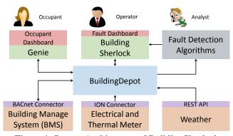
Figure 1. System Architecture of BuildingSherlock
