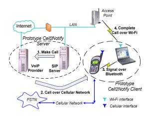
Figure 5: Our prototype implementation of Cell2Notify. We implement the Cell2Notify server as a combination of a commonly available SIP Proxy and an Internet- based VoIP gateway. We emulate a smartphone using a combination of a cellphone that communicates with a Wi-Fi equipped laptop using Bluetooth.
