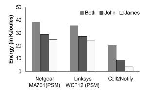
Figure 7: Energy consumption using two cards, with and without Cell2Notify for three different users. Cell2Notify saves more energy for lighter usage patterns.
