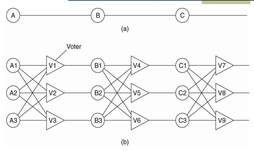
Triple modular redundancy in a circuit (b) A,B,C are circuit elements and V\* are voters
