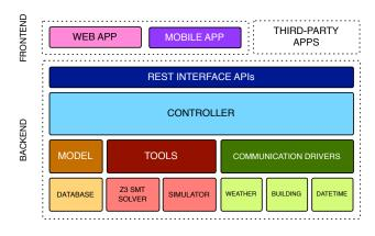
Figure 4: BuildingRules System Architecture
