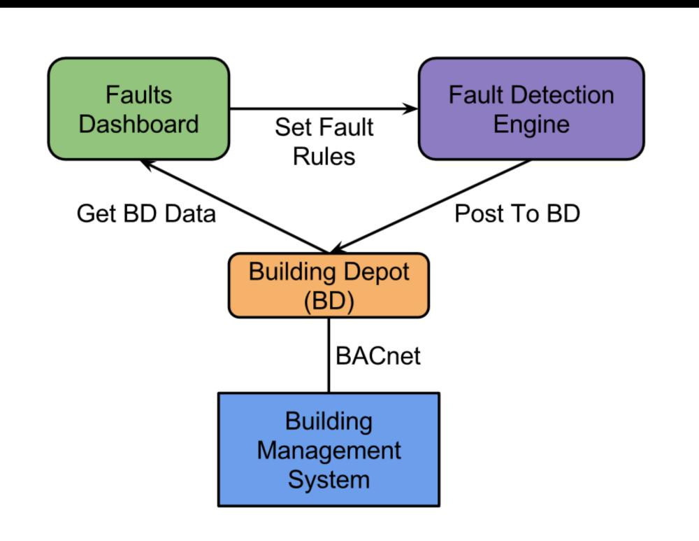
System Architecture of BuildingSherlock. The system is designed as a RESTful web service for ease of access, application development and scalability
